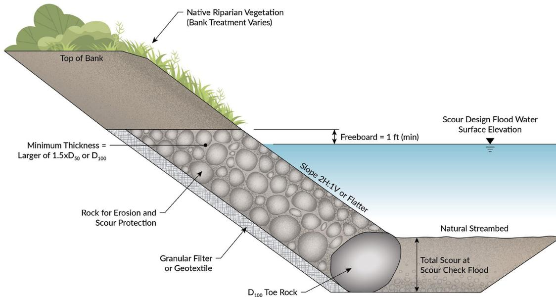
The filter material acts as a transition between the native soil and the rock, preventing the piping of fines through the voids of the rock structure while allowing relief of the hydrostatic pressure in the soil. Two types of filters are used: granular or geotextile. Filter materials are further described in the [Standard Specifications](#) and the [Geotechnical Design Manual](#). If the existing banks are similar to the filter material of sands and gravel, no filter layer may be needed.
