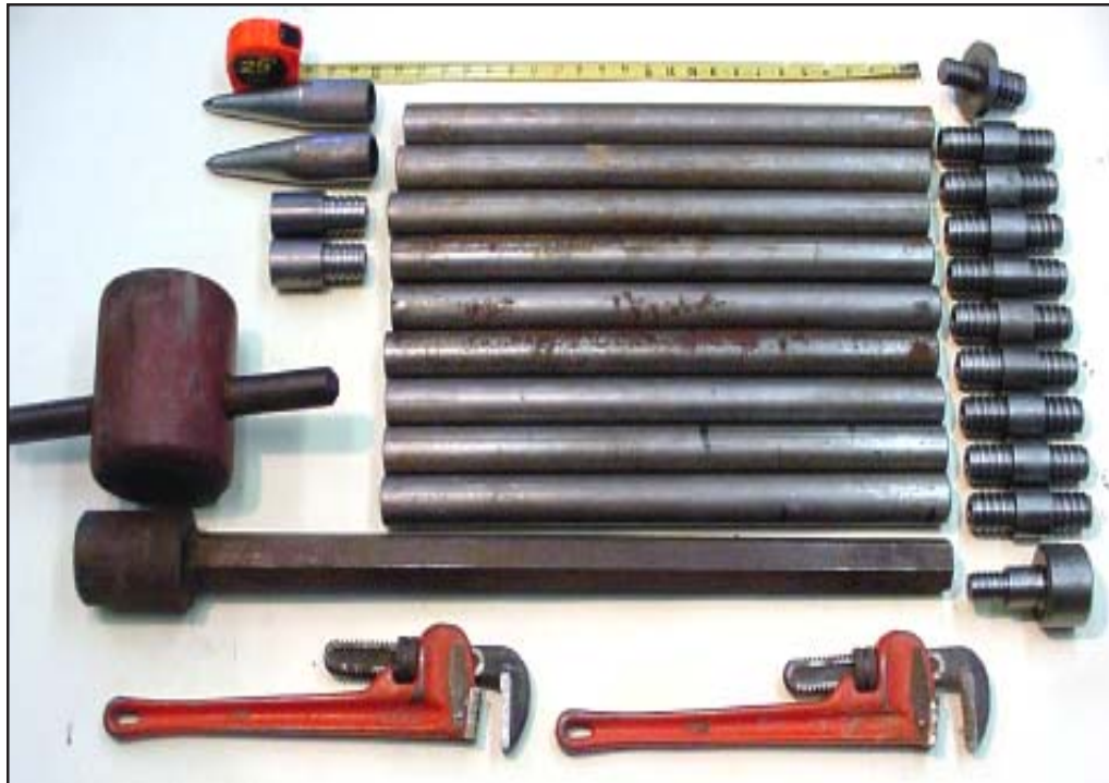
Porta-Pen equipment. Clockwise from the top left: tape measure above cone-shaped tips (2); 22.5-inch lengths (9); threaded coupling devices used to connect PP components (10); threaded coupler used to stop weight (1); falling-weight slide section above pipe wrenches (2); 35 lb. weight; and threaded coupling devices used with small cone tips (not shown).
