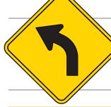
The horizontal alignment "CURVE" ahead advisory warning sign alerts motorists of the pending horizontal curvature in the roadway alignment.
