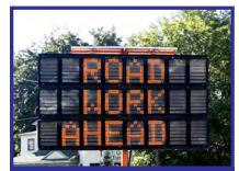
Variable Message Signs are one of the many ITS technologies used to anticipate and reduce congestion caused by highway work zones.
