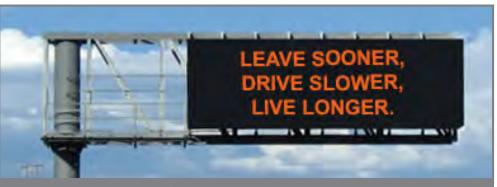
A VMS is an electronic traffic sign used on roadways to provide motorist with important information about traffic congestion, incidents, roadwork, travel times, special events or speed limits on a specific highway segment. They may also recommend alternative routes, limit travel speed, warn of duration and location of a problem or simply provide alerts or warnings.
