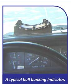
Banking is a tool used to determine if the existing speed limit of a curve can be driven safely and comfortably by most drivers. If it can not, a lower advisory speed limit sign and/or warning sign, such as TURN or CURVE
