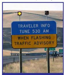
Commercial radio. both AM and FM are a ongoing source for weather, events and other information to drivers. HAR is used when there are upcoming concerns in the corridor. When the HAR sign flashes it is a notice to drivers that there is a radio message to
