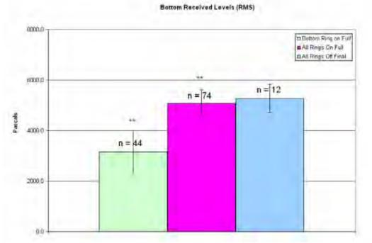
Figure 25: Pile 4, bottom average RMS received levels. Error bars represent one standard deviation. \* = Significant compared to bubbles off initial (p<0.05). \*\* Significant compared to bubbles off final (p<0.05)
