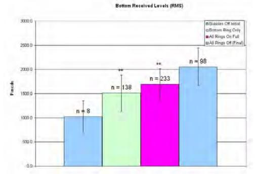
Figure 16: Pile 2, bottom average RMS received levels. Error bars represent one standard deviation. \* = Significant compared to bubbles off initial (p<0.05). \*\* Significant compared to bubbles off final (p<0.05)
