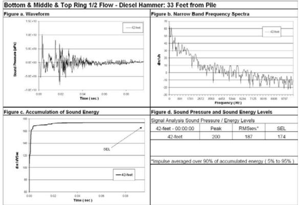
Figure 59 Waveform Analysis for Pile Number 1, 42-feet Deep (bottom), 33-Feet from Pile, Bottom, Middle, and Top Ring ½ Flow.
