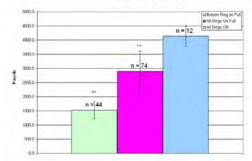
Figure 24: Pile 4, midwater average RMS received levels. Error bars represent one standard deviation. \* = Significant compared to bubbles off initial (p<0.05). \*\* Significant compared to bubbles off final (p<0.05)
