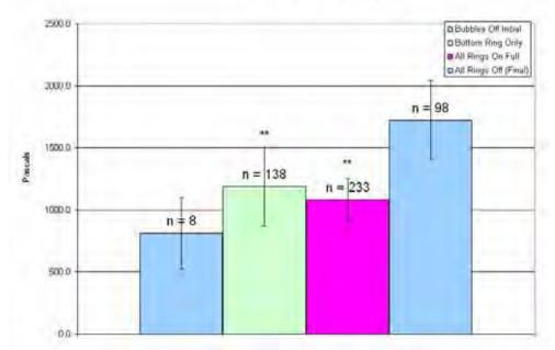
Figure 15: Pile 2, midwater average RMS received levels. Error bars represent one standard deviation. \* = Significant compared to bubbles off initial (p<0.05). \*\* Significant compared to bubbles off final (p<0.05)
