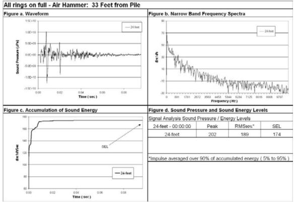
Figure 72 Waveform Analysis for Pile Number 2, 24-Feet Deep, 33-Feet from Pile, All Rings On Full.
