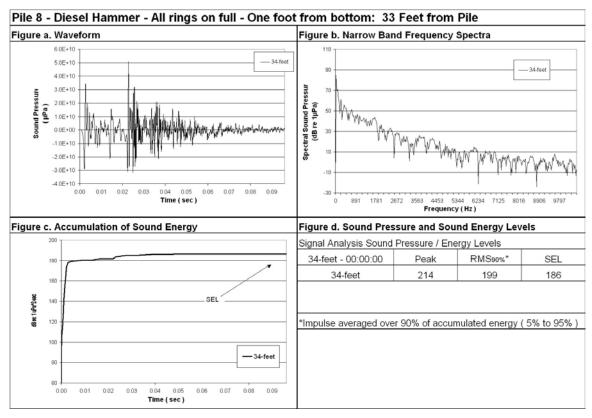
Figure 109: Waveform Analysis for Pile Number 8, 34-Feet Deep (Bottom), 33-Feet from Pile, All Rings On Full.
