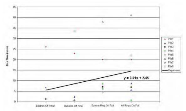
Figure 44. Rise times for each bottom received level peak pile strike with linear regression line
