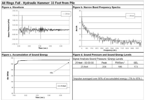
Figure 80 Waveform Analysis for Pile Number 3, 25-feet Deep, 33-Feet from Pile, All Rings Full.
