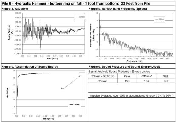
Figure 97: Waveform Analysis for Pile Number 6, 33-Feet Deep (Bottom), 33-Feet from Pile, Bottom Ring On Full.
