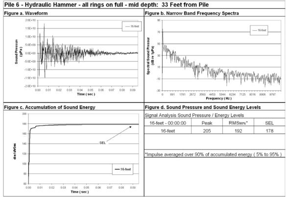
Figure 98: Waveform Analysis for Pile Number 6, 16-Feet Deep, 33-Feet from Pile, All Rings On Full.
