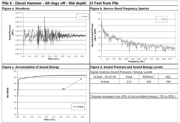
Figure 110: Waveform Analysis for Pile Number 8, 14-Feet Deep, 33-Feet from Pile, All Rings Off.
