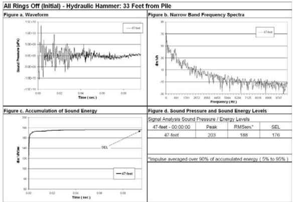
Figure 77 Waveform Analysis for Pile Number 3, 47-feet Deep (bottom), 33-Feet from Pile, All Rings Off.
