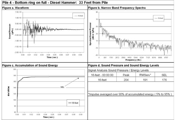
Figure 84: Waveform Analysis for Pile Number 4, 16-Feet Deep, 33-Feet from Pile, Bottom Ring On Full.
