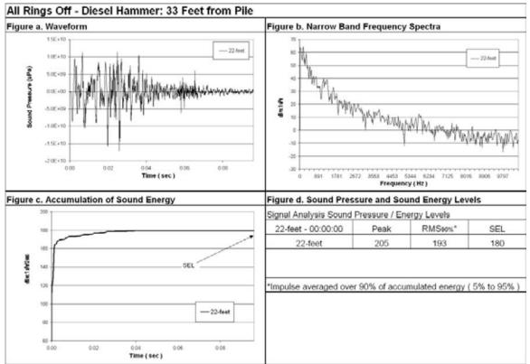
Figure 52: Waveform Analysis for Pile Number 1, 22-Feet Deep, 33-Feet from Pile, All Rings Off.
