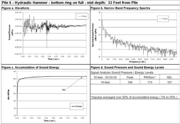
Figure 96: Waveform Analysis for Pile Number 6, 16-Feet Deep, 33-Feet from Pile, Bottom Ring On Full.
