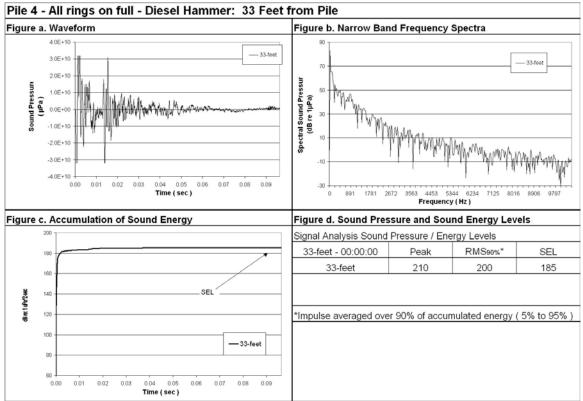
Figure 87: Waveform Analysis for Pile Number 4, 33-Feet Deep (Bottom), 33-Feet from Pile, All Rings On Full.
