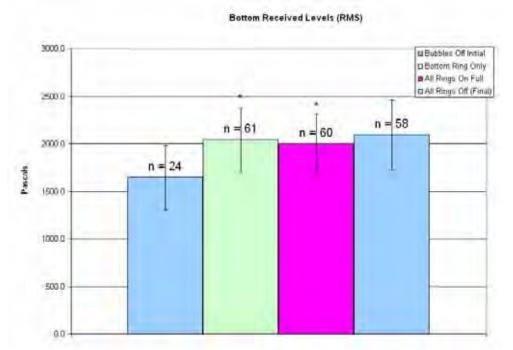
Figure 20: Pile 3, bottom average RMS received levels. Error bars represent one standard deviation. \* = Significant compared to bubbles off initial (p<0.05). \*\* Significant compared to bubbles off final (p<0.05)
