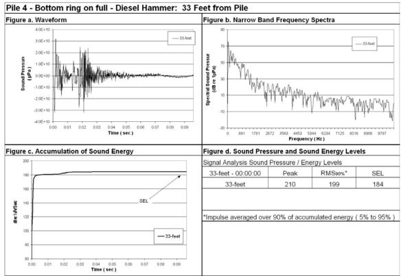
Figure 85: Waveform Analysis for Pile Number 4, 33-Feet Deep (Bottom), 33-Feet from Pile, Bottom Ring On Full.
