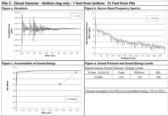
Figure 91: Waveform Analysis for Pile Number 5, 33-feet Deep (Bottom), 33-Feet from Pile, Bottom Ring On Full.
