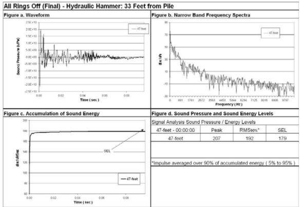
Figure 83 Waveform Analysis for Pile Number 3, 47-feet Deep (Bottom), 33-Feet from Pile, All Rings Off (Final).
