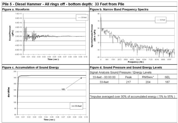
Figure 95: Waveform Analysis for Pile Number 5, 33-Feet Deep (Bottom), 33-Feet from Pile, All Rings Off.
