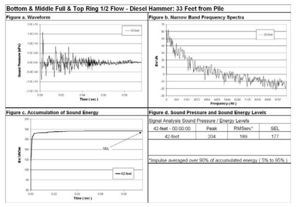
Figure 63 Waveform Analysis for Pile Number 1, 42-feet Deep (bottom), 33-Feet from Pile, Bottom and Middle Ring Full, Top Ring ½ Flow
