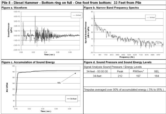
Figure 107: Waveform Analysis for Pile Number 8, 34-Feet Deep (Bottom), 33-Feet from Pile, Bottom Ring on full.
