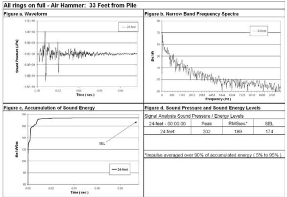
Figure 70 Waveform Analysis for Pile Number 2, 24-Feet Deep, 33-Feet from Pile, Bottom Ring On Full.
