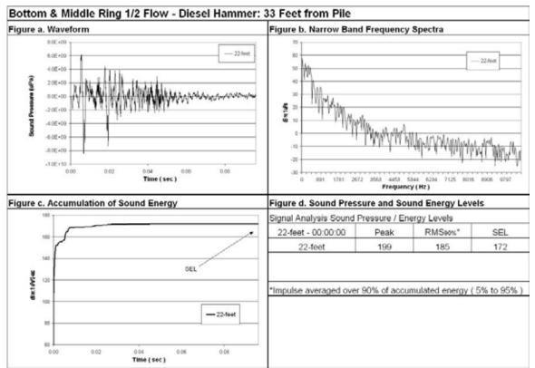
Figure 56: Waveform Analysis for Pile Number 1, 22-feet Deep, 33-Feet from Pile, Bottom and Middle Ring ½ Flow.
