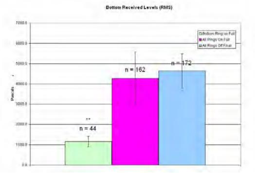
Figure 33. Pile 6, bottom average RMS received levels. Error bars represent one standard deviation. \* = Significant compared to bubbles off initial (p<0.05). \*\* Significant compared to bubbles off final (p<0.05
