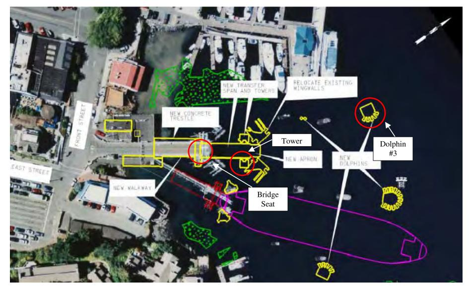
Figure 1: Location of Underwater Noise Monitoring at Friday Harbor. There were three 24-inch piles monitored at Dolphin #3, three 24-inch piles monitored at the Bridge Seat, and two 30-inch piles monitored at the Tower.
