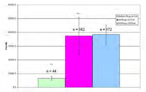
Figure 31. Pile 6, bottom average peak received levels. Error bars represent one standard deviation. \* = Significant compared to bubbles off initial (p<0.05). \*\* Significant compared to bubbles off final (p<0.05)
