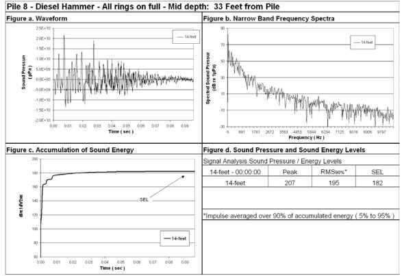
Figure 108: Waveform Analysis for Pile Number 8, 14-Feet Deep, 33-Feet from Pile, All Rings On Full.
