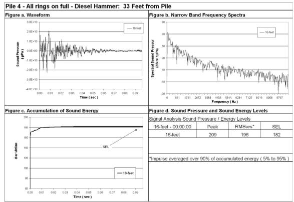
Figure 86: Waveform Analysis for Pile Number 4, 16-Feet Deep, 33-Feet from Pile, All Rings On Full.
