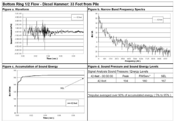
Figure 55: Waveform Analysis for Pile Number 1, 42-feet Deep (Bottom), 33-Feet from Pile, Bottom Ring ½ Flow.
