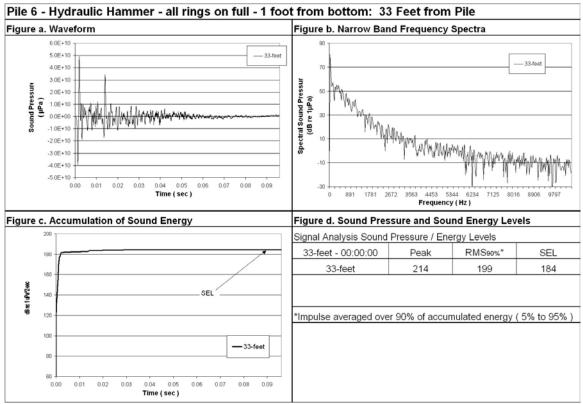
Figure 99: Waveform Analysis for Pile Number 6, 33-Feet Deep (Bottom), 33-Feet from Pile, All Rings On Full.
