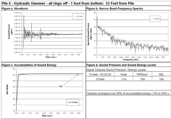
Figure 101: Waveform Analysis for Pile Number 6, 33-Feet Deep (Bottom), 33-Feet from Pile, All Rings Off.
