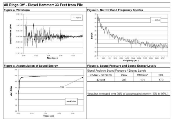
Figure 53: Waveform Analysis for Pile Number 1, 42-feet (Bottom), 33-Feet from Pile, All Rings Off.
