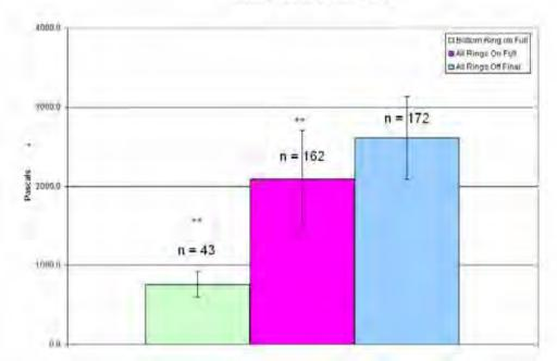
Figure 32. Pile 6, midwater average RMS received levels. Error bars represent one standard deviation. \* = Significant compared to bubbles off initial (p<0.05). \*\* Significant compared to bubbles off final (p<0.05)
