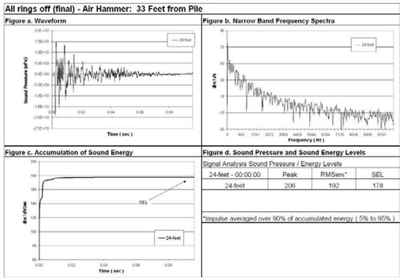
Figure 74 Waveform Analysis for Pile Number 2, 24-Feet Deep, 33-Feet from Pile, All Rings Off (Final).
