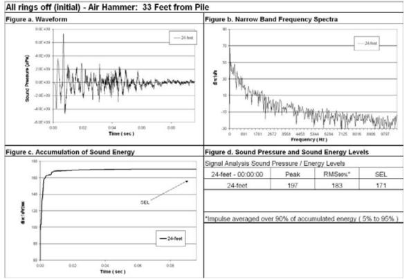
Figure 68: Waveform Analysis for Pile Number 2, 24-Feet Deep, 33-Feet from Pile, All Rings Off.
