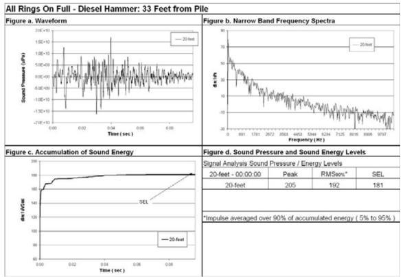
Figure 104: Waveform Analysis for Pile Number 7, 20-Feet Deep, 33-Feet from Pile, All Rings On Full.
