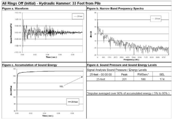
Figure 76 Waveform Analysis for Pile Number 3, 25-feet Deep, 33-Feet from Pile, All Rings Off (Initial).
