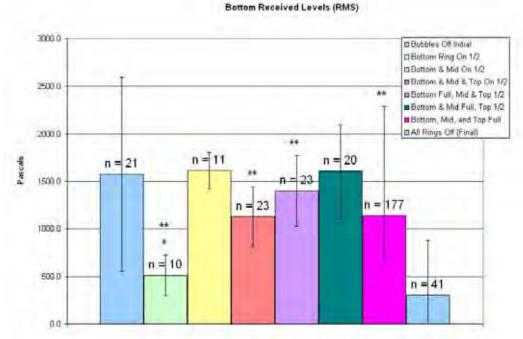
Figure 10: Pile 1, bottom average RMS received levels. Error bars represent one standard deviation. \* = Significant compared to bubbles off initial (p<0.05). \*\* Significant compared to bubbles off final (p<0.05).
