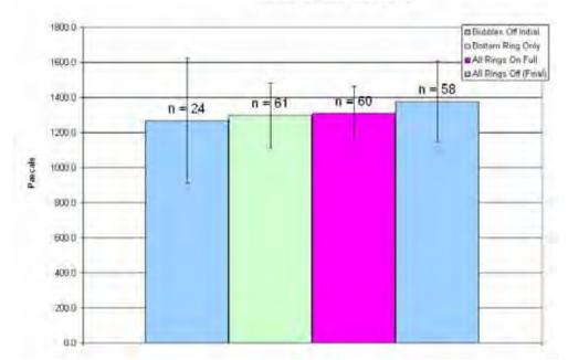
Figure 19: Pile 3, midwater average RMS received levels. Error bars represent one standard deviation. \* = Significant compared to bubbles off initial (p<0.05). \*\* Significant compared to bubbles off final (p<0.05)
