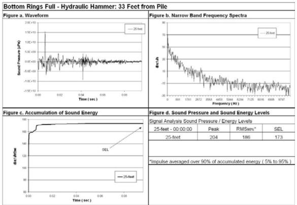
Figure 78 Waveform Analysis for Pile Number 3, 25-feet Deep, 33-Feet from Pile, Bottom Ring On Full.
