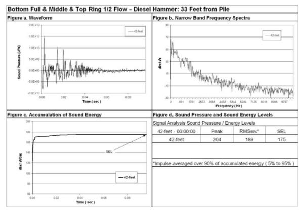
Figure 61 Waveform Analysis for Pile Number 1, 42-feet Deep (bottom), 33-Feet from Pile, Bottom Ring Full, Middle, and Top Ring ½ Flow.
