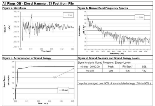
Figure 88: Waveform Analysis for Pile Number 4, 16-Feet Deep, 33-Feet from Pile, All Rings Off.
