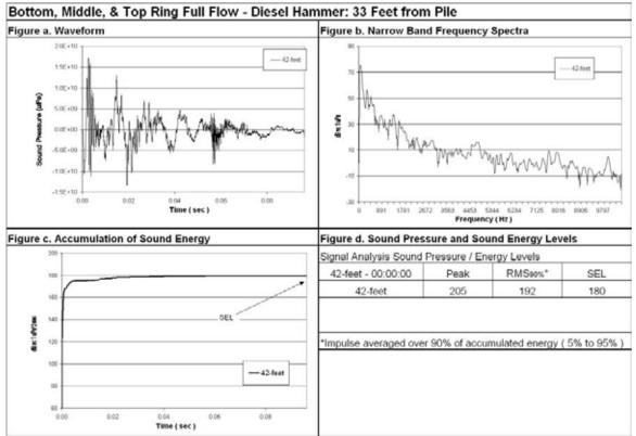
Figure 67 Waveform Analysis for Pile Number 1, 42-feet Deep (bottom), 33-Feet from Pile, All Rings Off (Final).
