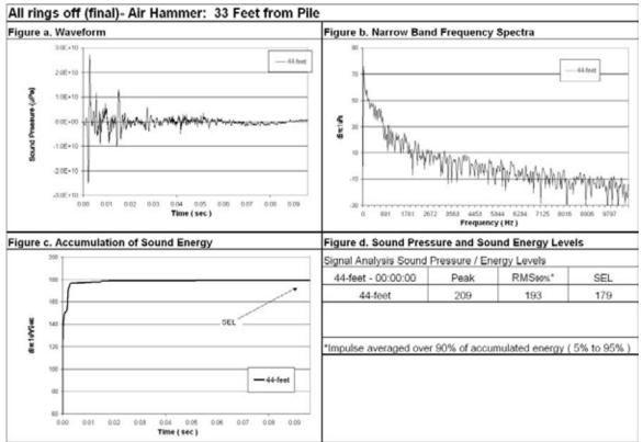
Figure 75 Waveform Analysis for Pile Number 2, 44-Feet Deep (Bottom), 33-Feet from Pile, All Rings Off (Final).
