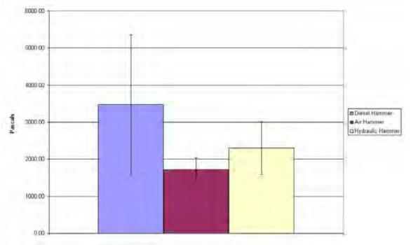
Figure 47. Average RMS midwater received values for each hammer type, all bubble rings off. Error bars are ± one standard deviation
