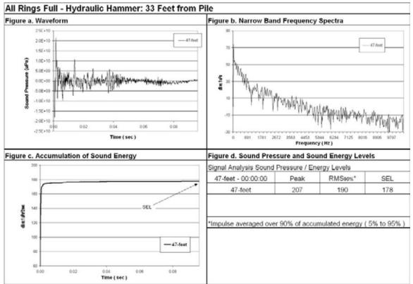
Figure 81 Waveform Analysis for Pile Number 3, 47-feet Deep (Bottom), 33-Feet from Pile, All Rings Full.
