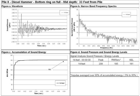
Figure 106: Waveform Analysis for Pile Number 8, 14-Feet Deep, 33-Feet from Pile, Bottom Ring on full.
