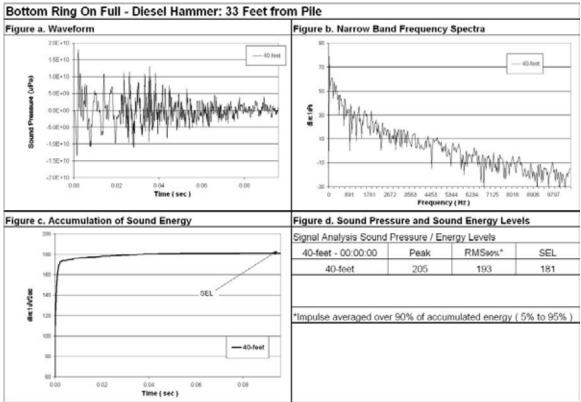
Figure 103: Waveform Analysis for Pile Number 7, 40-Feet Deep (Bottom), 33-Feet from Pile, Bottom Ring On Full.
