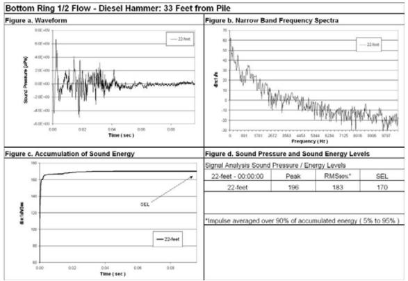
Figure 54: Waveform Analysis for Pile Number 1, 22-Feet Deep, 33-Feet from Pile, Bottom Ring <sup>1</sup>/<sub>2</sub> Flow.
