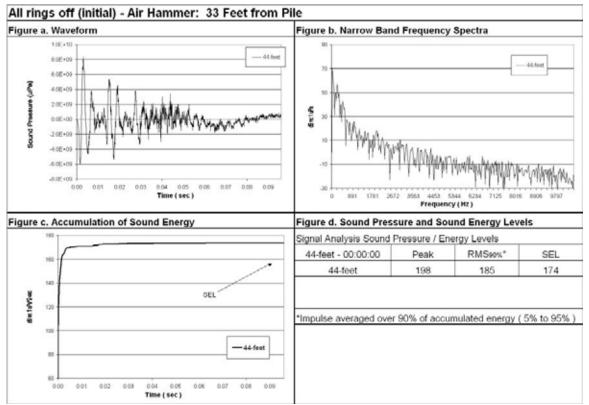
Figure 69: Waveform Analysis for Pile Number 2, 44-Feet Deep (bottom), 33-Feet from Pile, All Rings Off.
