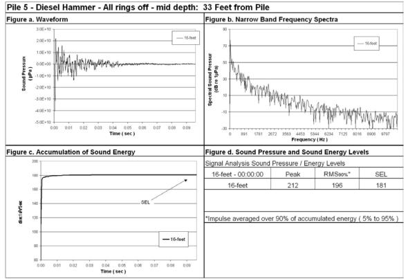
Figure 94: Waveform Analysis for Pile Number 5, 16-Feet Deep (Bottom), 33-Feet from Pile, All Rings Off.
