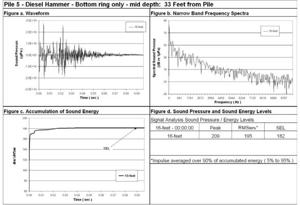
Figure 90: Waveform Analysis for Pile Number 5, 16-feet Deep, 33-Feet from Pile, Bottom Ring On Full.
