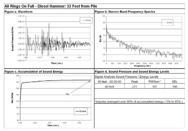
Figure 105: Waveform Analysis for Pile Number 7, 40-Feet Deep (Bottom), 33-Feet from Pile, All Rings On Full.
