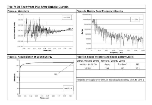
Figure 51: Results of Sound Pressure Levels with Bubble Curtain.
