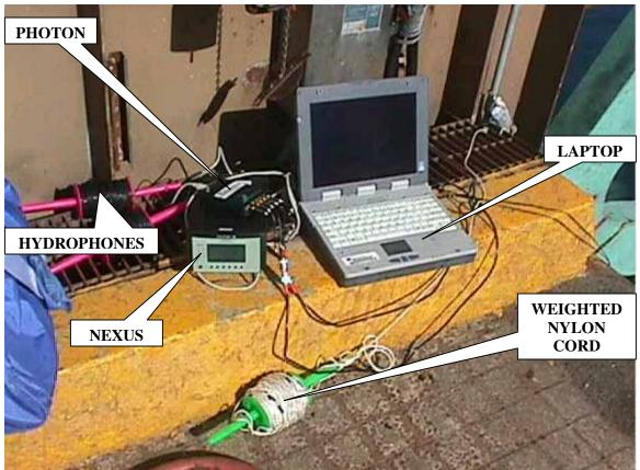
Figure 2: Underwater Sound Level Measurement Equipment
