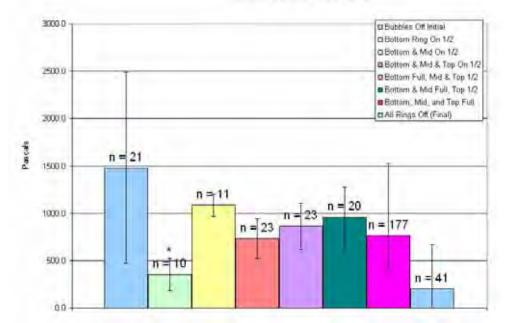
Figure 9: Pile 1, midwater average RMS received levels. Error bars represent one standard deviation. \* = Significant compared to bubbles off initial (p<0.05). \*\* Significant compared to bubbles off final (p<0.05).
