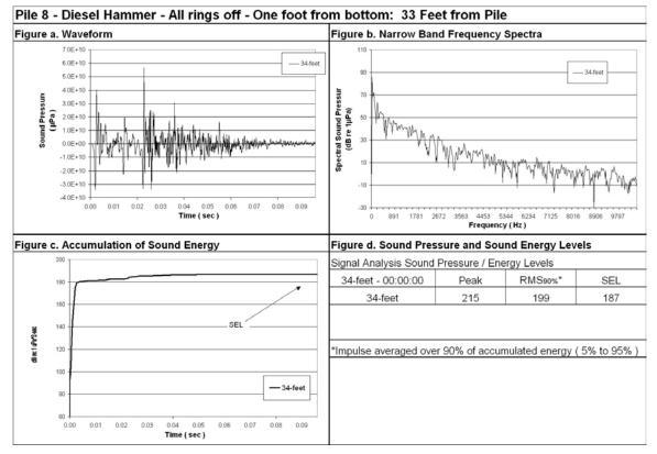
Figure 111: Waveform Analysis for Pile Number 8, 34-Feet Deep (Bottom), 33-Feet from Pile, All Rings Off.
