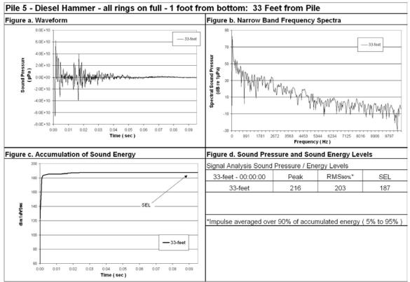
Figure 93: Waveform Analysis for Pile Number 5, 33-Feet Deep (Bottom), 33-Feet from Pile, All Rings On Full.
