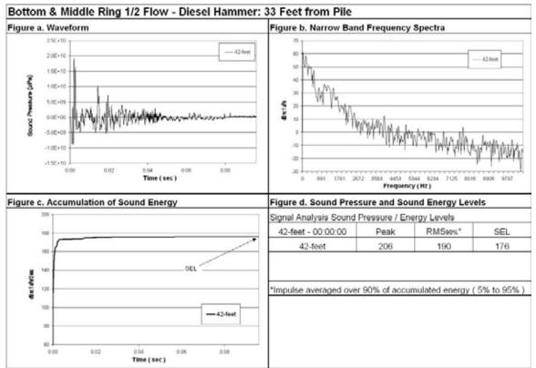
Figure 57: Waveform Analysis for Pile Number 1, 42-feet Deep (Bottom), 33-Feet from Pile, Bottom and Middle Ring <sup>1</sup>/<sub>2</sub> Flow.
