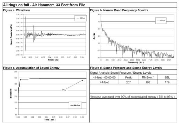
Figure 73 Waveform Analysis for Pile Number 2, 44-Feet Deep (Bottom), 33-Feet from Pile, All Rings On Full.
