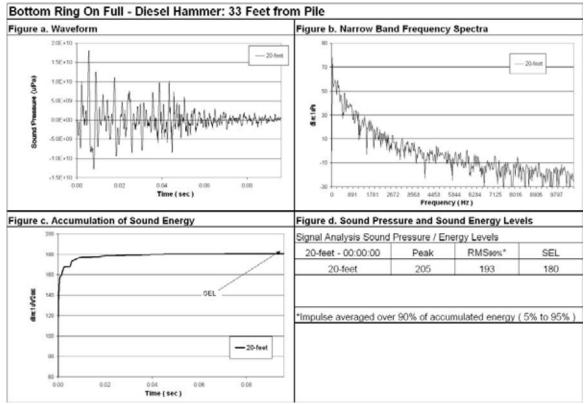
Figure 102: Waveform Analysis for Pile Number 7, 20-Feet Deep, 33-Feet from Pile, Bottom Ring On Full.
