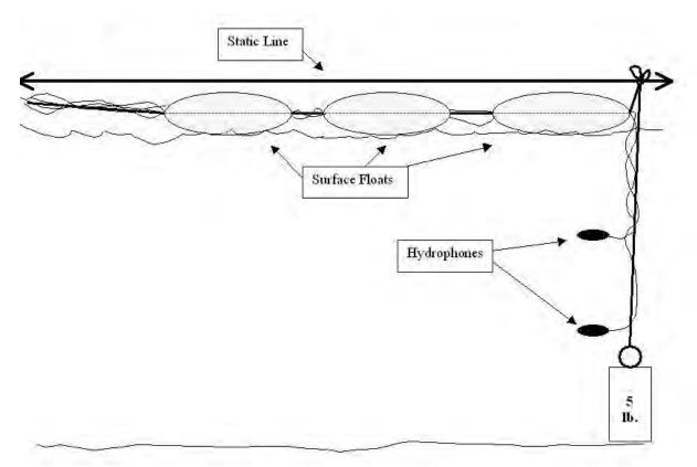
Figure 3: Hydrophone Weight and Float System
