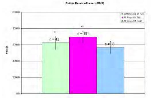
Figure 29. Pile 5, bottom average RMS received levels. Error bars represent one standard deviation. \* = Significant compared to bubbles off initial (p<0.05). \*\* Significant compared to bubbles off final (p<0.05)
