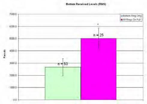
Figure 38. Pile 7, bottom average RMS received levels. Error bars represent one standard deviation. \* = Significant compared to bottom ring on only (p<0.05).
