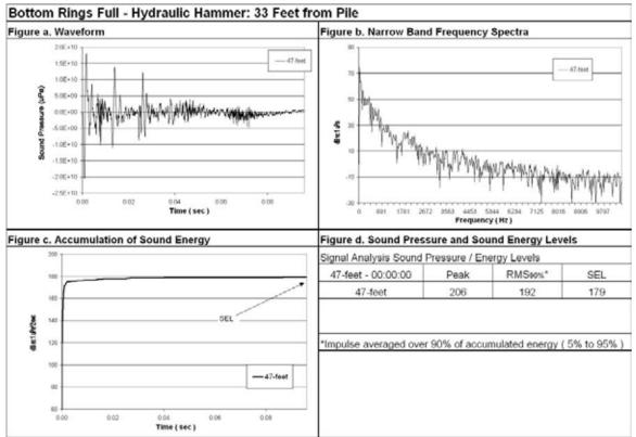
Figure 79 Waveform Analysis for Pile Number 3, 47-feet Deep (Bottom), 33-Feet from Pile, Bottom Ring On Full.
