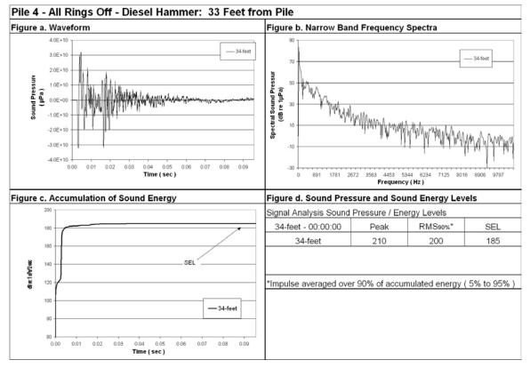
Figure 89: Waveform Analysis for Pile Number 4, 34-Feet Deep (Bottom), 33-Feet from Pile, All Rings Off.
