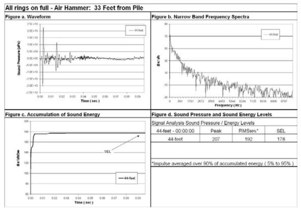
Figure 71 Waveform Analysis for Pile Number 2, 44-Feet Deep (bottom), 33-Feet from Pile, Bottom Ring On Full.
