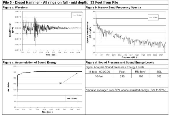
Figure 92: Waveform Analysis for Pile Number 5, 16-Feet Deep, 33-Feet from Pile, All Rings On Full.
