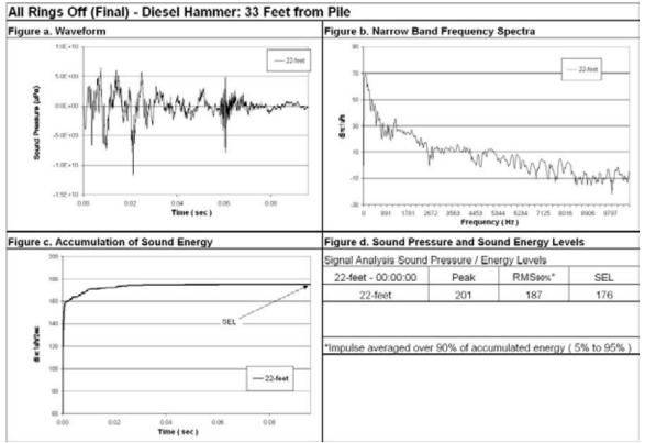
Figure 66 Waveform Analysis for Pile Number 1, 22-feet Deep, 33-Feet from Pile, All Rings Off (Final).
