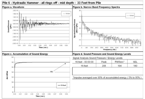
Figure 100: Waveform Analysis for Pile Number 6, 16-Feet Deep, 33-Feet from Pile, All Rings Off.
