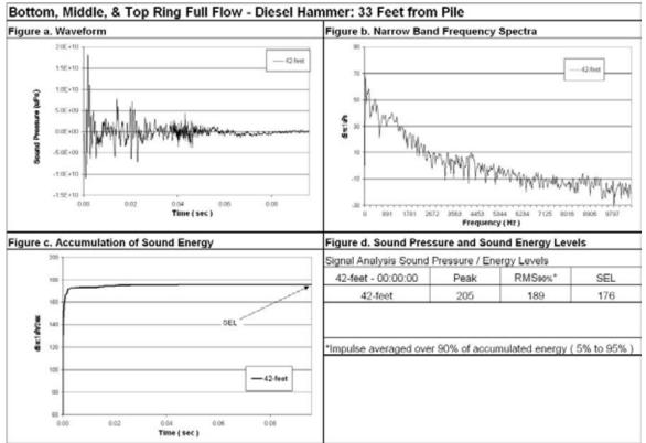
Figure 65 Waveform Analysis for Pile Number 1, 42-feet Deep (bottom), 33-Feet from Pile, Bottom, Middle, and Top Ring Full Flow
